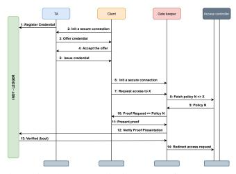
Fig. 3: First phase communication process of a read request.
