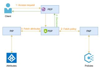
Fig. 1: An overview of the architecture of XACML.
