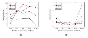
Fig. 6: Throughput and latency of DecideRead in terms of block size and batch timeout (bt).
